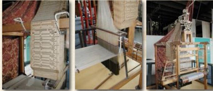
Joseph Jacquard, Punch Card Controlled Loom
